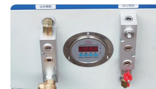
Quick water pressure testing
